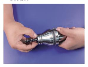
**5** Lock (Arrow pointing up and down) with a torque wrench. 用扭力扳手鎖緊(箭頭標上下對齊)。
